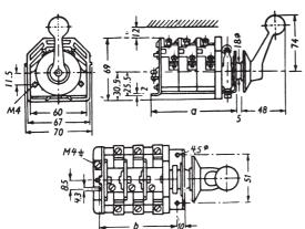
\* Minimum clearance from metal parts (to be increased to 18 mm in case of 3LAO 204-5YA)
