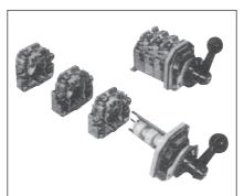
Switches with red ball handle or red machine handle can be supplied on request. The handle engages with the indicating dial by means of serrations. After the cap nut has been loosened, the handle can be fixed in any one of 16 different positions. In this way, the position of the handle can be adjusted to the mounting requirements in each individual case.
